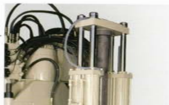
BMC進料 BMC Material Loading
