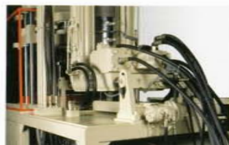
液壓式BMC擠壓進料裝置 BMC Material Loading Unit
